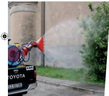
The perfect and **uniform micronization** produced using a unique type of pneumatic nozzle, with a large diameter (4 mm), and **fade-free functionality**, **no wear**, no clogging, no maintenance.
