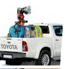
The perfect and **uniform micronization** produced using a unique type of pneumatic nozzle, with a large diameter (4 mm), and **fade-free functionality**, **no wear**, **no clogging**, **no maintenance**.
