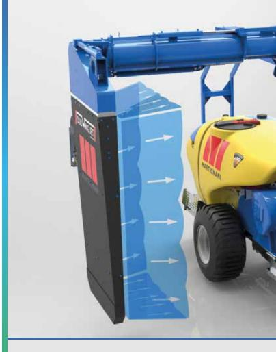
The Duo Wing Jet can be considered the first and only mist blower that recovers the product by combining the electrostatic attraction between the vegetation and the electrically charged micro-droplets (+ -) with that of two special protective screens with an air-cushion that extends beyond their edge; without any recycling of the pesticide mixture and not only with 99% anti-drift but also with no chemical residues on fruits, grapes, wine etc.
